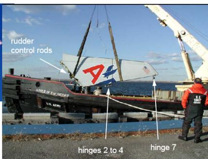
Separated Fin being recovered, control rods and hinges are marked on the photo
