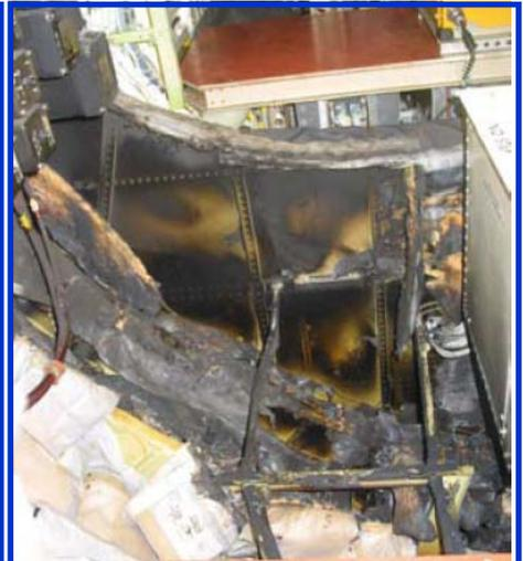
Figure 3. Burnt aircraft structure & insulation blankets located directly below P200 power panel (viewed looking down & aft; the floor panel has been removed)
